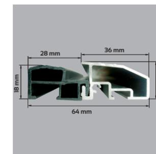
ALUMINIUM THRESHOLD WITH THERMAL INSERT
