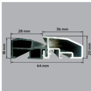
ALUMINIUM THRESHOLD WITH THERMAL INSERT
