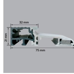
ENERGO THRESHOLD WITH THERMAL INSERT
